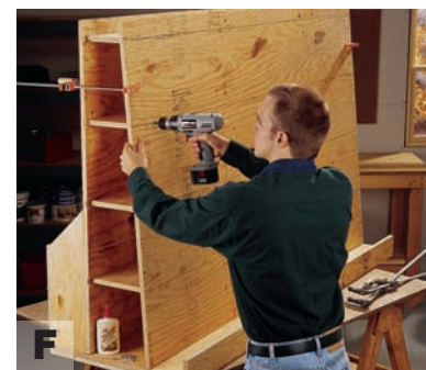
F Draw centerlines for the shelves on the angled side, then fasten the angled side to the shelves with glue and screws. Screw up through the bottom to attach the angled side from below.
