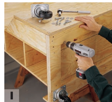
I Fasten the clamp holders to scrap blocking, and screw the blocking to the end of the cart with 1-1/2-in. wood screws. Keep the slots aligned between the holders so the clamps will hang straight.
