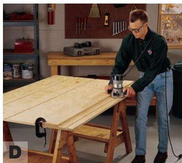
**D** Cut shelf dadoes in the vertical side with a router and straightedge guide. Pull the router toward you as you make each cut, being careful to hold the router base tight against the straightedge as you work.
