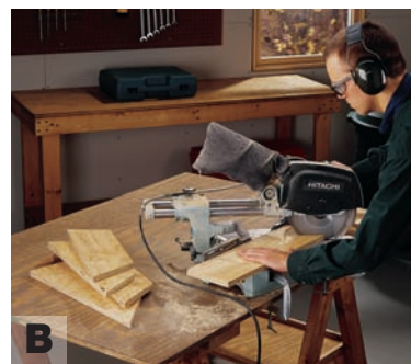
B Cut the angled ends of the dividers. A power miter saw makes this task quick and easy, once you've established the cutting angle. You can also make these cuts with a jig saw, table saw or circular saw.
