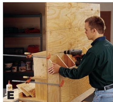
**E** Fasten the shelves to the vertical side with glue and screws. Support the shelves with scrap-wood spacers. Insert the square edge of the shelves into the dadoes, and keep the beveled edges facing up.
