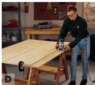
D Cut shelf dados in the vertical side with a router and straightedge guide. Pull the router toward you as you make each cut, being careful to hold the router base tight against the straightedge as you work.
