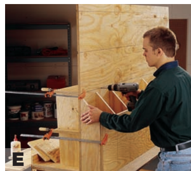
E Fasten the shelves to the vertical side with glue and screws. Support the shelves with scrap-wood spacers. Insert the square edge of the shelves into the dados, and keep the beveled edges facing up.
