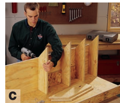
C Glue and screw the dividers to the tall edge with 1-1/2-in. wood screws. Use scrap-wood spacers inserted between the dividers to establish divider spacing.
